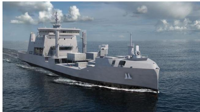
HMNZS Aotearoa will be a world-first naval "Enviroship", with Hyundai using the Rolls-Royce Enviroship concept design under licence. The design incorporates a new wave-piercing hull, which reduces resistance and lowers fuel use, while its combined diesel electric and diesel propulsion plant has lower fuel emissions than older vessels.
